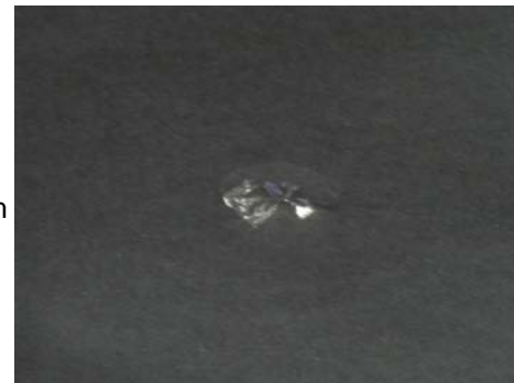
50 μm thick film of spider silk protein
