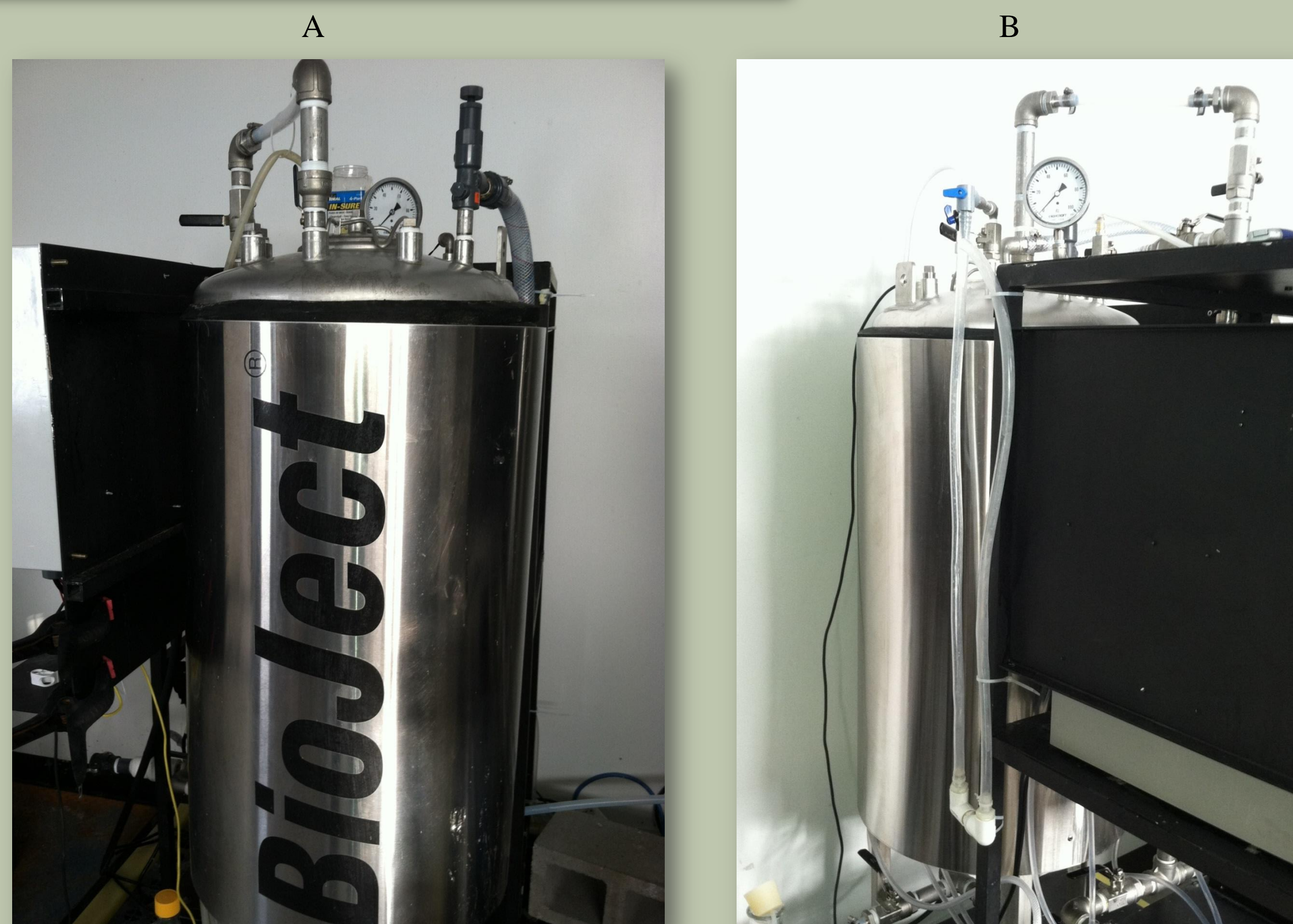
A pair of modified 110L bioreactors for pilot scale ABE production from algae biomass. A) Pretreatment reactor to lyse algae cells for increased ABE yields. B) The ABE bioreactor for producing acetone, butanol, and ethanol from algae.
