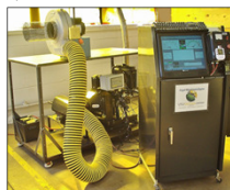
2) Figure 2. Dynamometer and emissions setup with a Kubota Z482 to test the fuels.
