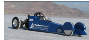
7) Figure 7. Initial streamliner design used for 2012 season
