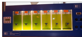
Figure 6. Jar tests were used for chemical testing.
