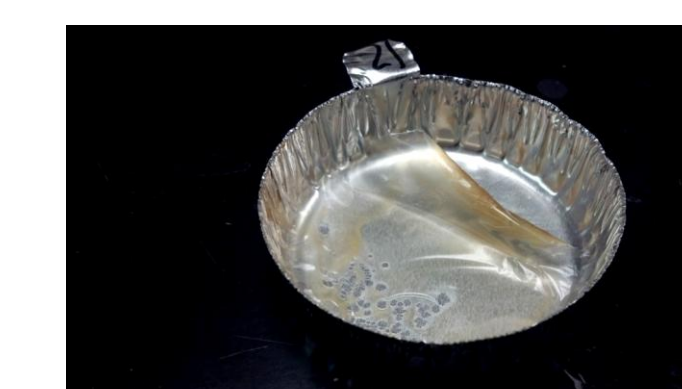
Sample of PHB extracted from E. coli biomass using Propylene Carbonate.
