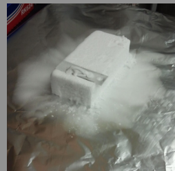
Figure 4: Preserving stained biofilm samples in embedding medium using dry ice.
