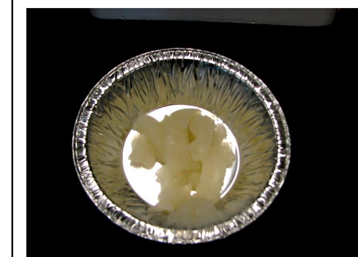
3 Solvent phase collected (Propylene Carbonate), cooled, and mixed with Ethanol to precipitate PHB
