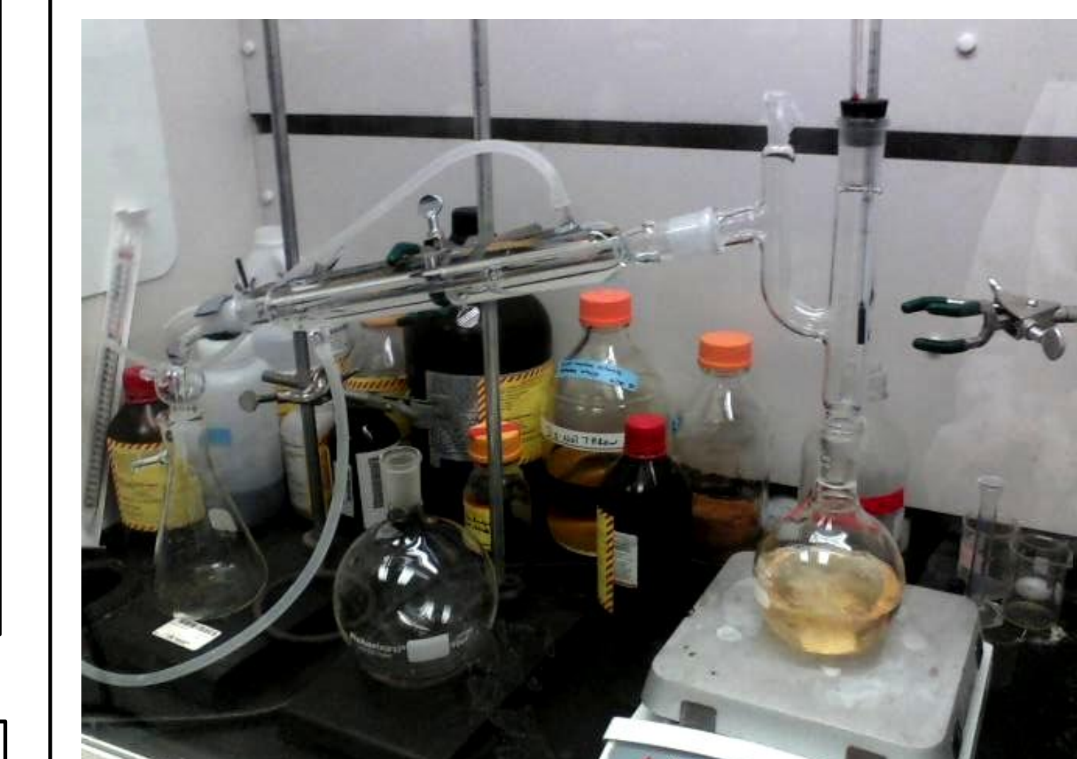
Distillation apparatus to recover Propylene Carbonate and Ethanol from waste stream
