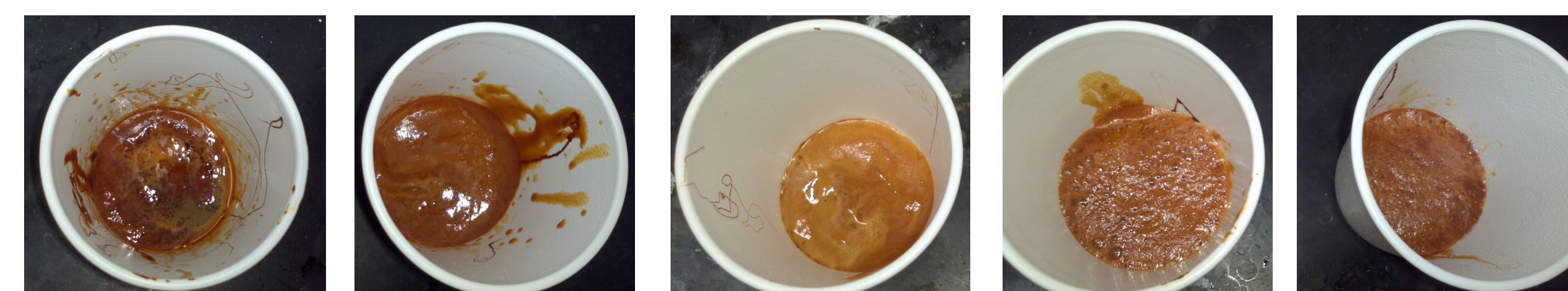
Figure 6. Foams produced using bio-oil with constant quantity of surfactant and increasing amounts of water, from left to right.
