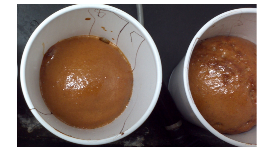
Figure 7. Foams produced using 1.3 eq of blowing agent and 0.7 eq of surfactants result in foams with low density and higher compressibility.
