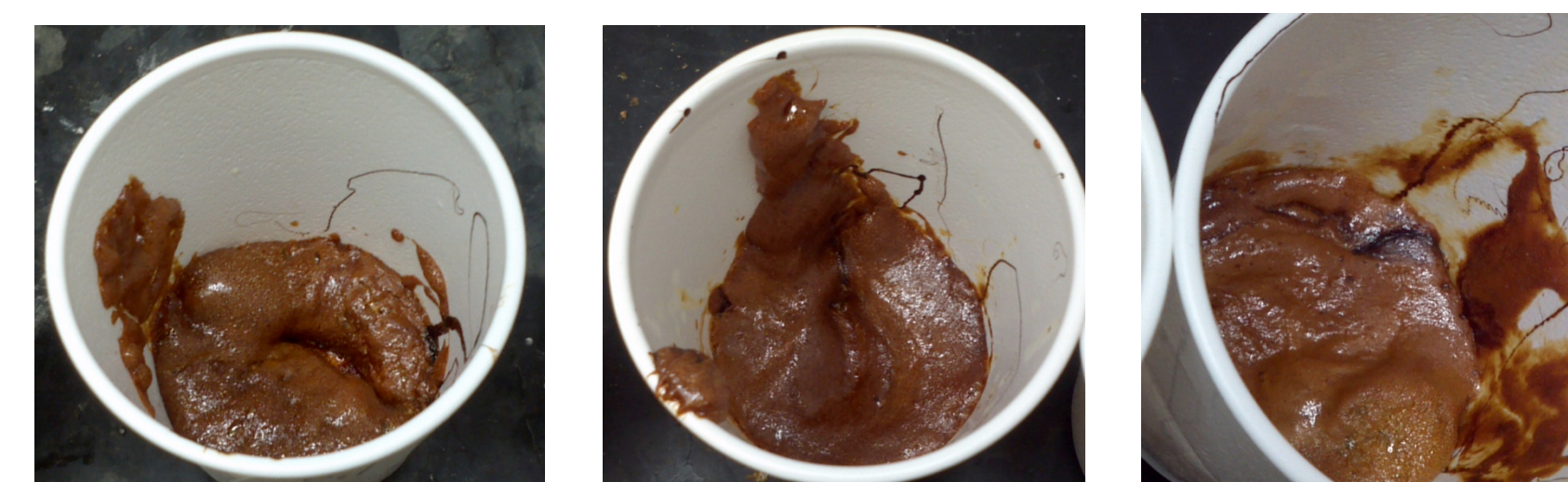
Figure 5. Increasing amounts of surfactant do not affect the quality of foam, but consistently produce brittle foams.
